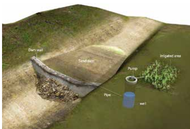
Figure 23: The increase in sand sediments on the original riverbed caused by the construction of a sand storage dam: a diagram (left) and a real-life example (right). Source: Pixinit Studios. Photo: J. de Trinchieria.
