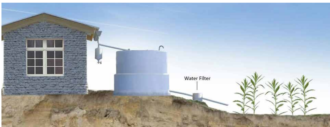
Figure 44: A roof catchment system coupled with a surface water tank. Source: Pixiniti Studios.
