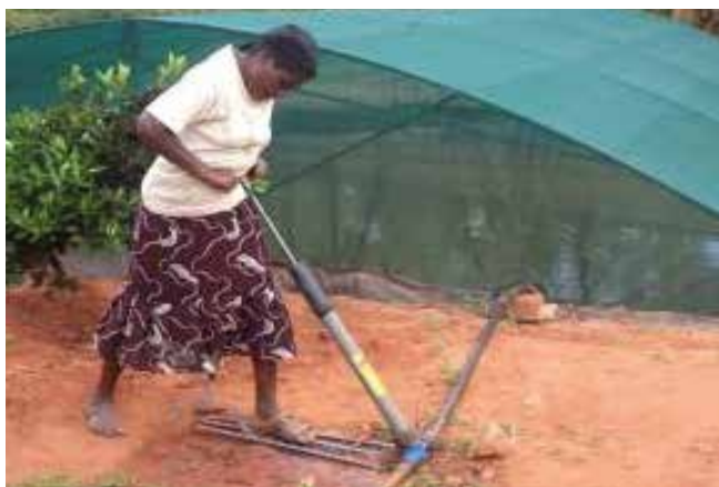
Figure 60: Hip-pump (left) for lifting water from a farm pond into a drip irrigation system (right) in Makueni, Kenya. Photos: S. Ngigi.
