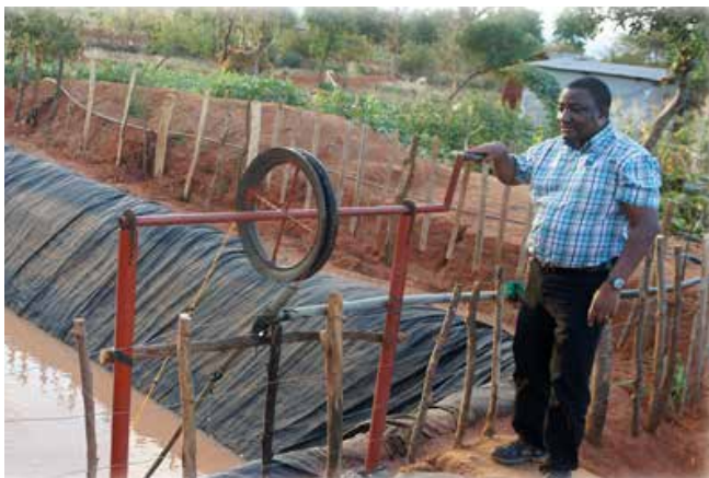
Figure 58: Operation of the rope and washer pump. Photo: A. Oduor.
